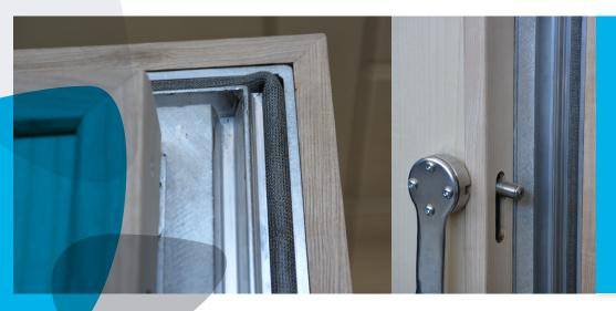
RF door contains three pistons that rotate 90° to create a tight seal. Using a Z-shaped frame and two military grade gaskets that never need to be replaced, this door does not require periodic maintenance.
